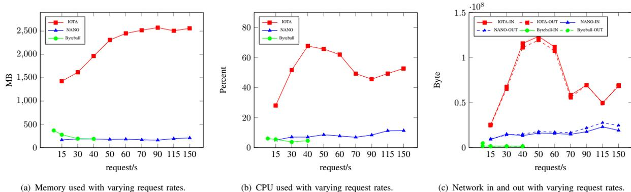
Fig. 6. CPU, memory and network flow with 8 clients and 8 nodes.
