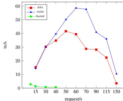
Fig. 3. Throughput with 8 clients and 8 (DAG network) nodes.
