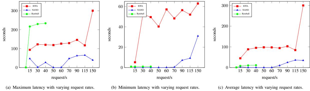
Fig. 4. Latency with 8 clients and 8 nodes.
